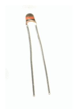
$$T = \frac{1}{\frac{1}{298.16 \,\text{K}} + \frac{1}{B} \ln \left(\frac{R}{R_{25}}\right)},$$
