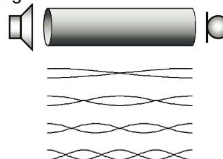
**FIGURE 6.** The sketch of the experiments for the measurement of the acoustic modes of a tube.
