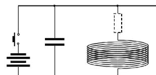
**FIGURE 4.** The sketch of the RLC circuit used in the demonstration.
