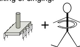
**FIGURE 5.** The Pneumobelt consists of an elastic tube around the waist and a pressure sensor.
